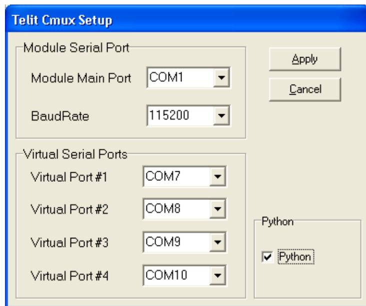
Set the *Module Main Port* as the real COM port you have available (e.g. COM1 in the figure), check the Python box and then select the Apply button.
