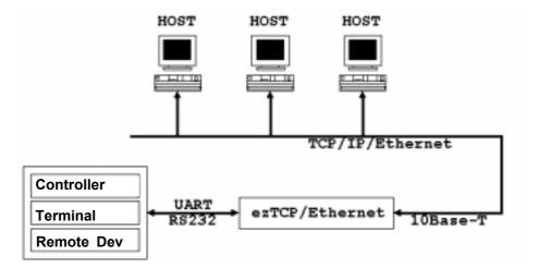
If a host computer (hereafter a host) is connected to the TCP port of ezTCP over an Ethernet network, the serial port of the DTE is connected virtually to the TCP port of the host. Then, ezTCP will function as an intermediate device between the serial port and the TCP port.
