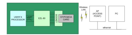
EZL-80 is a small-sized, modular product that provides TCP/IP communication through IEEE802.11b (wireless LAN) among the ezTCP product group and requires 16-bit PCMCIA card or CF card interface and a corresponding wireless LAN card.
