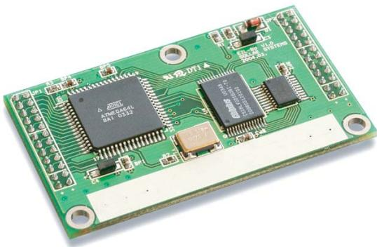
small module TCP/IP converter
