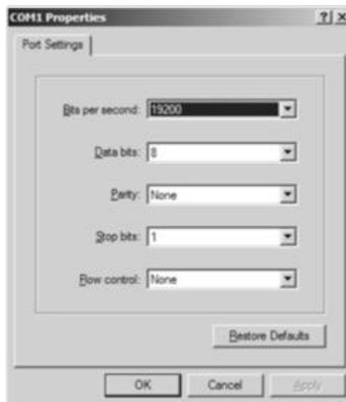
**Figure 9 Hyper Terminal Set Up**
