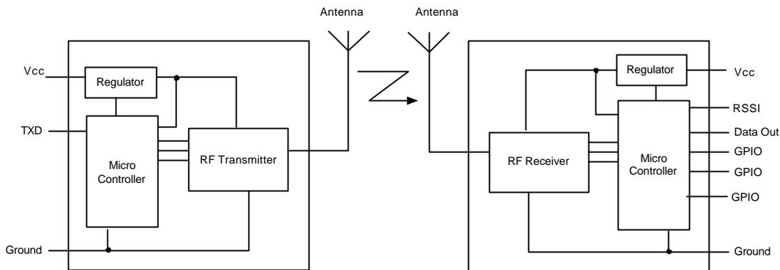
**Figure 1 Transmitter & Receiver Block Diagram**
