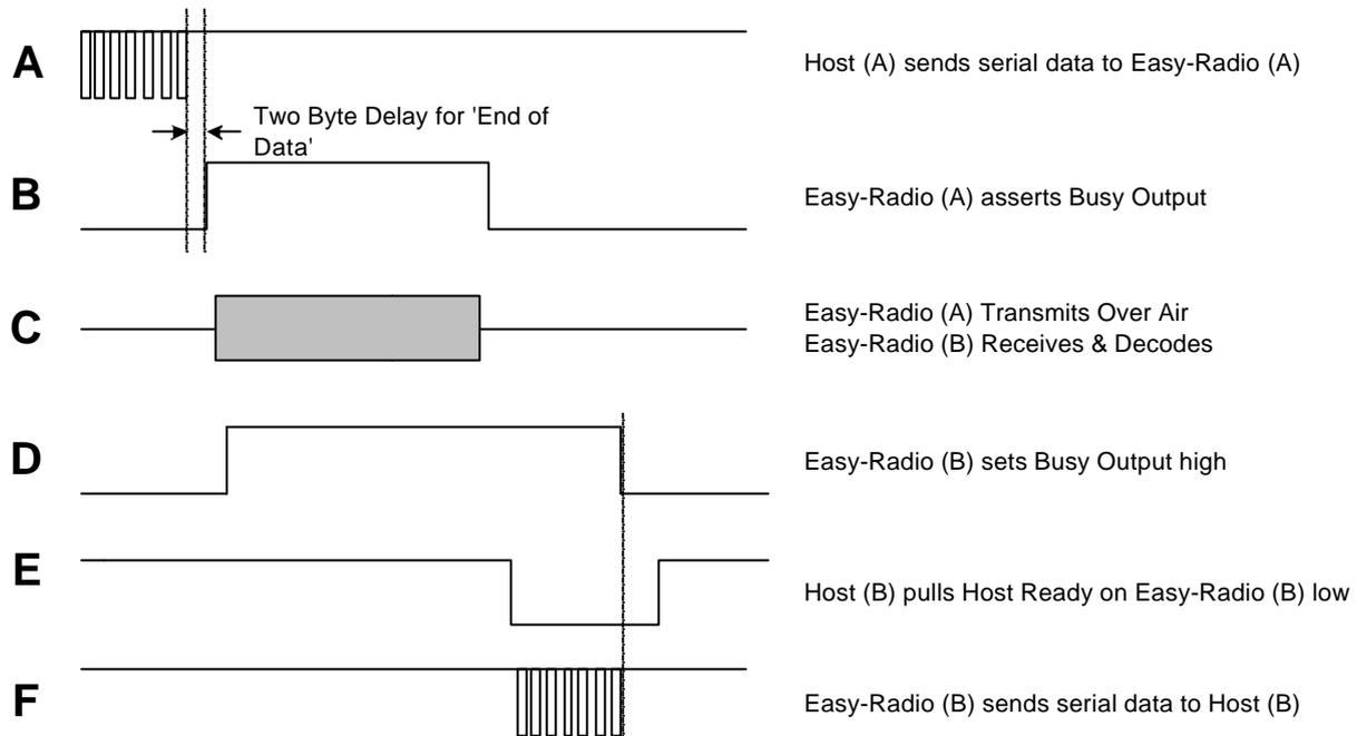
**Figure 6 Timing Diagram**
