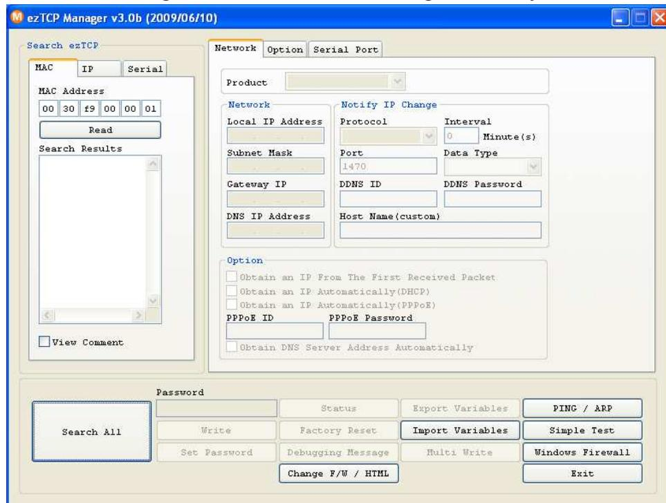
ezManager communicates UDP broadcast and its UDP ports are 50005 and 50006. Port number 50005 is for setting and port number 50006 is for debugging. If you use any firewall function, the ports have to be opened.
