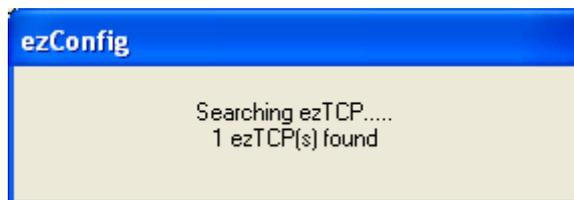
√ *It is impossible to use ezConfig, if EZCFG check box is disabled. This function can be re-enabled in ISP mode.*
