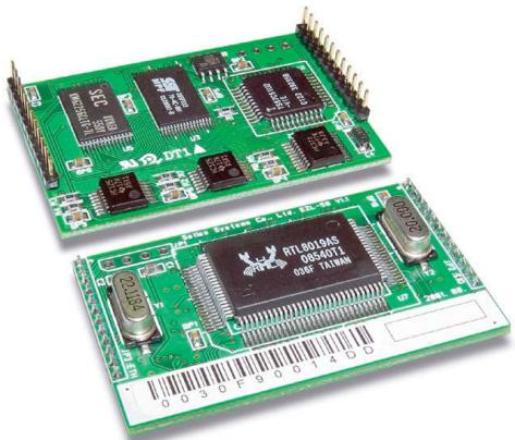
small module TCP/UDP/IP converter
